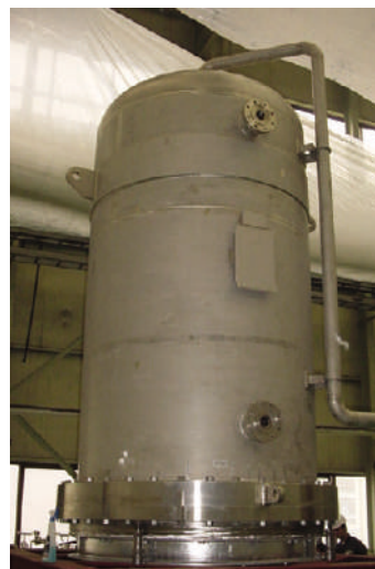
• CVD Reactor Featuring Pressure Vessel Technology
